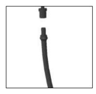
11 Push the Drop Tubes into the Barbed Adapters (on the main LDPE Pipe).
